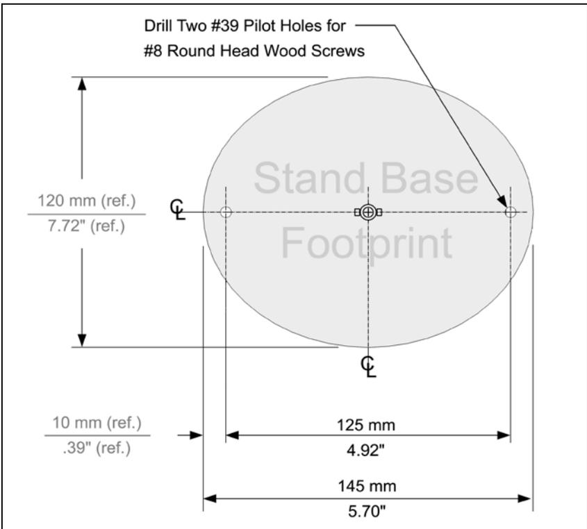
*Figure 15. Stand Base Hole Pattern (Not to Scale)*
