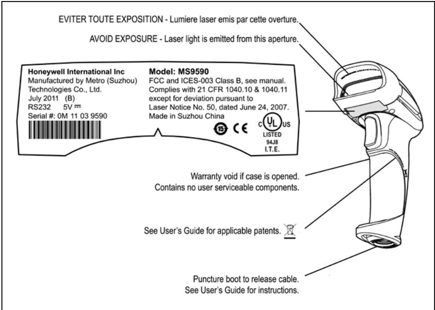
Figure 4. Molded Text and Serial Number Label
